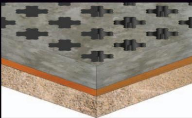
Pour concrete as per specifications and smooth flush to top of the CM100 forms. Melt the top thin section to reveal the void space.
